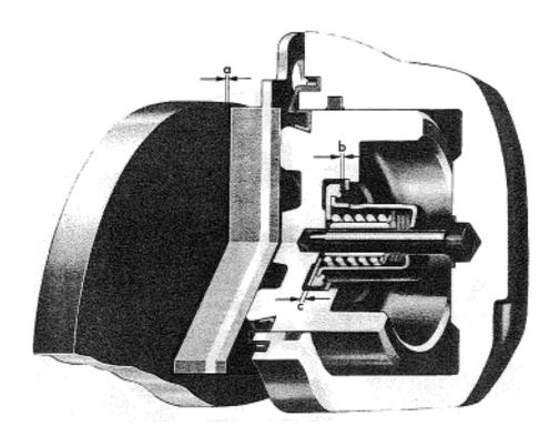
Clearance a is the clearance between friction pads and brake disc.
