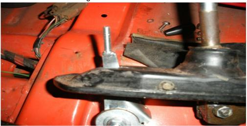
Install the bracket for the push rod
