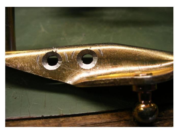
Wrong (!!) make sure that the nuts are on the back side
