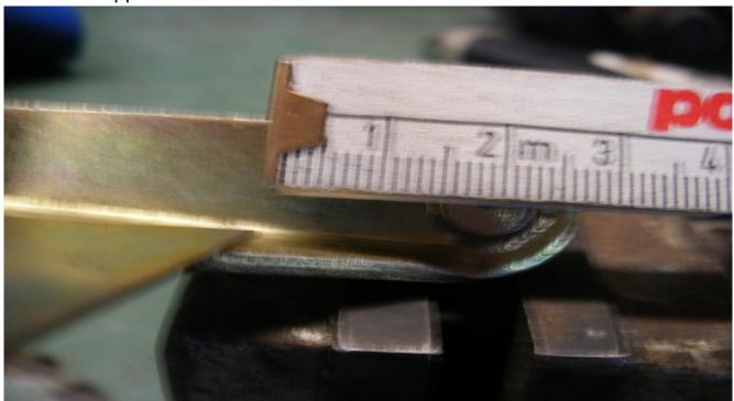
Mark two points on the enhancement and drill these with the 5mm drill Transfer the holes between the markers on the accelerator arm and drill it also with the 5mm drill. After this lowering the bores like the pictures show
