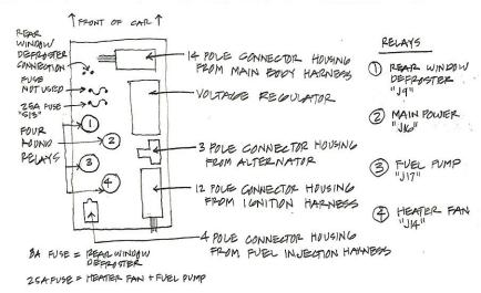
VOLTAGE REGULATOR / ENGINE BAY RELAY BOARD
