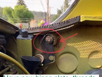
Have new hinge plate, threads and bolt ready to replace damaged left rear trunk hinge all others OK.
