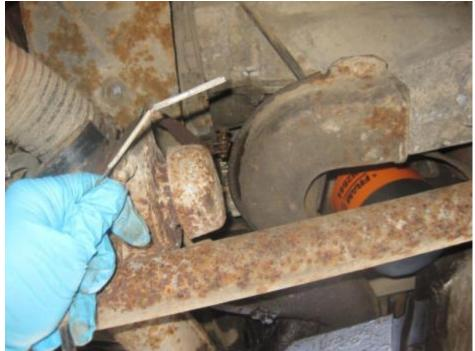
33. Loop the cables toward the front of the car so that they are out of the way.
