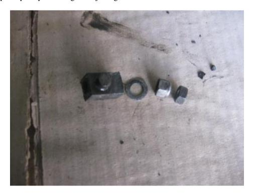
Then remove the nut and clip that retains the clutch cable pulley. I gently pried the cable from where it mounts with a screwdriver and fiddled with that clip thingy until it came loose.
