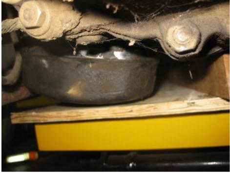
Here's a pic looking from the side showing how the 2 x 4 is under the rear supporting area of the crankcase.
