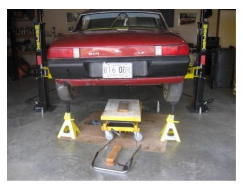
Here are some pictures from after the engine and transmission were dropped to illustrate how the 2 x 4 provides support while clearing the rear shifter housing and clutch pulley bracket.
