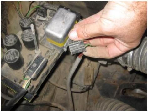
13. Don't forget to open the retaining tabs that hold the wires in place (check all applicable wires for these).
