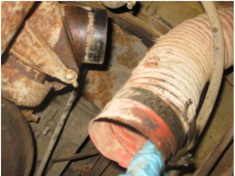
30. Disconnect the heater cable from each of the flapper boxes. Over the whole procedure, this was the most difficult component to take apart. The bolts were rusted on and it was difficult to counter hold the mechanism without breaking it. In the end I snapped one of the cables.
