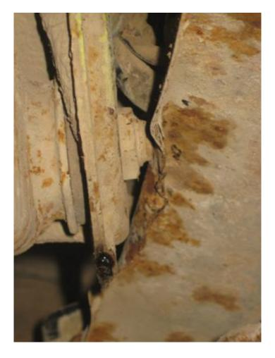
Ensure that the rear axles are not catching. The left one on mine needed to be fished through the wiring by the starter.
