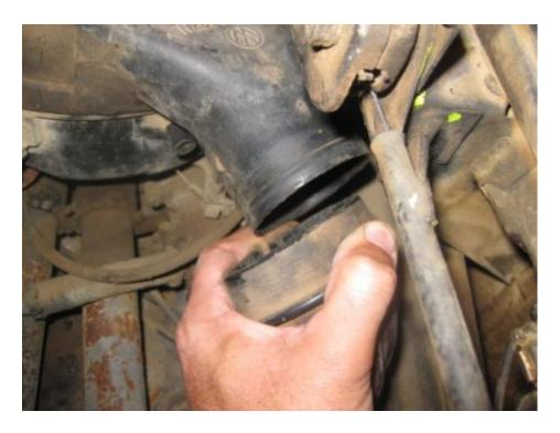
...and then remove the air cleaner housing from the engine compartment.
