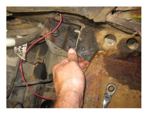
Then the fuel injection brain should wiggle out from its location.
