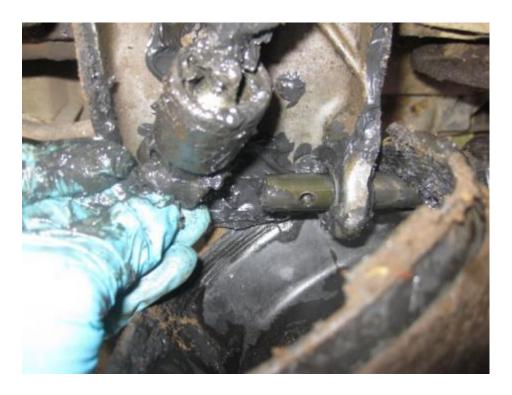
Wayne cautions not to lose the couplings because they can now slide off of the shaft. He also suggests to inspect the shifter bushings and replace as needed (see the Pelican article 914 shifting improvements). The front of the bar took some gentle persuasion with a large flathead screwdriver to get it off.
