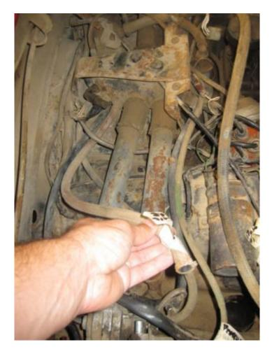
17. Disconnect the electrical connector and the line on the fuel pressure regulator.
