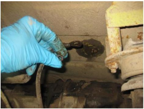
29. Move to the front of the engine and disconnect the lower heater hoses from each side of the car (there was only one hose on mine).
