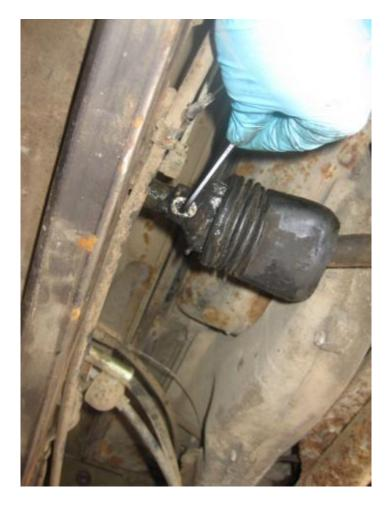
Inspect the cone screw to ensure it's in good condition.
