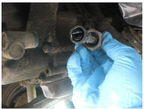
24. Disconnect the clutch cable. Wayne's instructions say to "start by loosening up the adjusting nut and removing the V-shaped piece at the end of the cable from the throw-out arm." I fumbled a bit with this trying to figure it out. The adjusting nut was a bit seized so I used one wrench to counterhold the cable.
