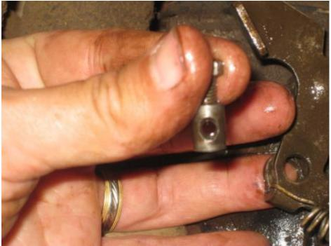
Next, lift the cable up and out of its mounting location under the bracket for the air cleaner. Mine was a little bit tight as it hadn't been removed in at least 30 years, but with some pressure it popped out.
