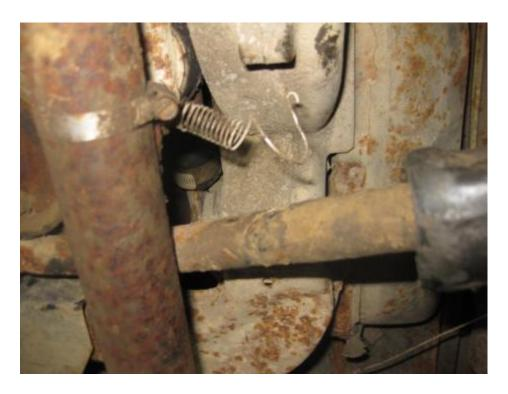
Then I fished the shifter bar through the engine bar and out it came.
