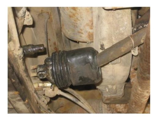
My car had a spring from the engine bar going around the shifter bar (doesn't look to be stock, nor is the engine bar!). So I disconnected the spring.
