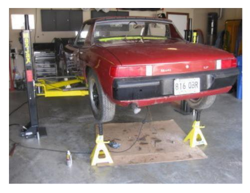
25. Hopefully your car isn't like this, but if it is and you choose to continue then pucker, while you hope that the back end doesn't fall off and land on you, and fish the speedometer and clutch cables through the engine bar.
