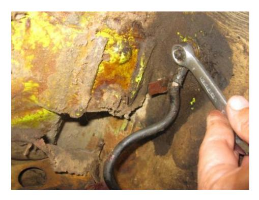
19. Disconnect the fuel injection computer from its mounting location on the firewall
