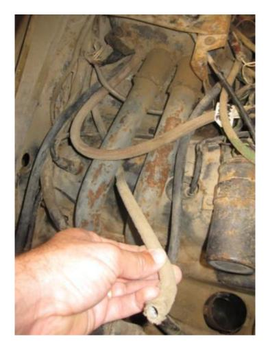
18. I don't recall seeing this step in Wayne's write-up, but disconnect the engine ground. I disconnected mine from the side of the car rather than the engine because I'm hoping to restore the car and will need to clean out the engine bay anyway.
