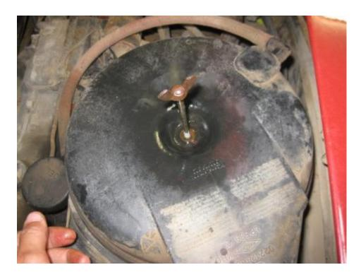
7. Before removing the air cleaner, disconnect the breather line that goes to the oil fill tube.
