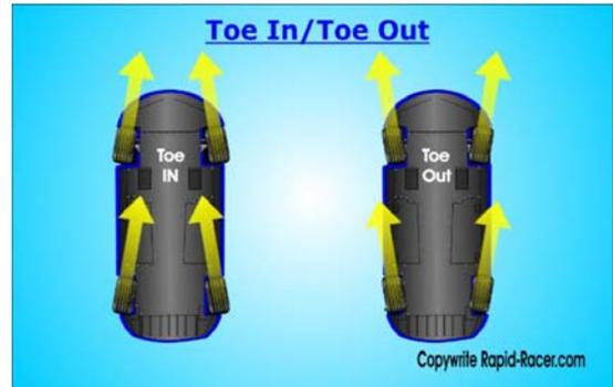
The toe setting are normally measured in degrees from the wheels' centerline, toe in is represented as negative degrees (-) and toe out is positive degrees (+).
