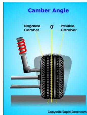
With any suspension adjustments and tuning, the best rewards will be achieved with a good baseline and small incremental changes for optimum results. Any camber angle adjustment will be positive up to a certain degree, until the settings have a negative impact on handling characteristics.
