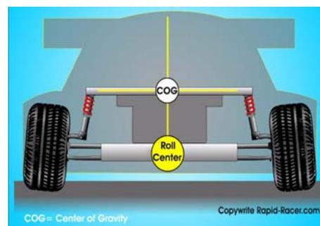
It is critical to understand that all acceleration, braking and lateral g-forces go through this point and the whole suspension system is set up and designed around this point.
