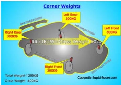
This is why static weight is so important to get right in the first place. As discussed in the static weight page, if we do find out we have a less than perfect weight distribution, it is possible to make suspension tuning adjustments to counter act these in balances. Sometimes the static weight might change due to off track diversion, will sequential damage or misalignments to the car.
