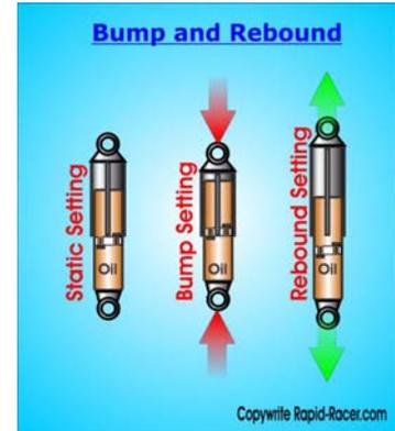
Shocks effectively help to dissipate any vertical movement in the suspension and keep the springs movements controlled, also they help the wheel keep full motion under different loads, while keeping the wheel in contact with the ground.
