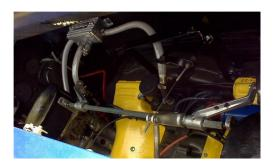
**Step 1** – Remove the drop arms from the carbs on both sides, and set the throttle plate in the closed position on each one –I back off the idle speed screw completely, then use a 0.005" feeler to set the clearance so the screw is not touching the stop.
