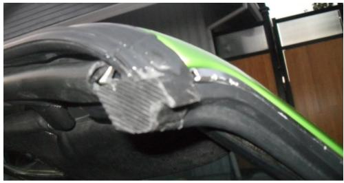
Note the new plugs were slightly longer than the old ones. I did use a set of the side targa roof seals that were cut slightly longer than OEM. These required me to trim about 1/8" off to fit properly
