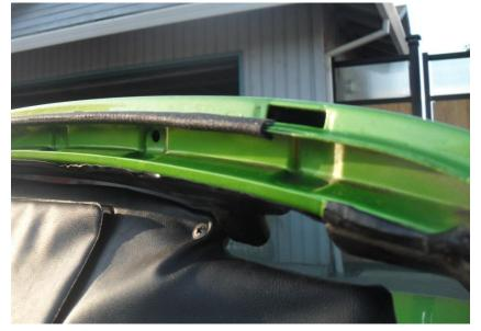
This seal is not glued on, it presses in place, it will be a firm fit. It will not go from corner to corner as it will need some relief to follow the contour of the top. The inner clip goes between the vents (as shown) it will not run all the way to the end as it need relief to make the contour without bulging.
