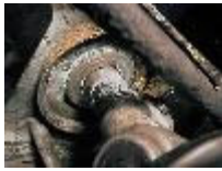
Figure 2: Firewall Shifter Rod Bushing
